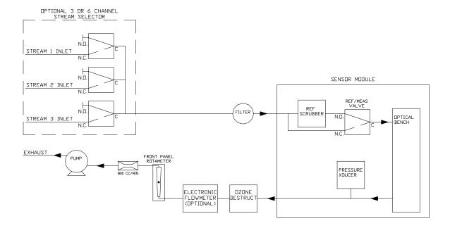
Figure 10-1: Pneumatic Diagram, 3 Stream Configuration
